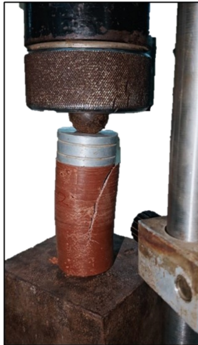
Figure 9. UCS test specimen undergoing unidirectional loading.
