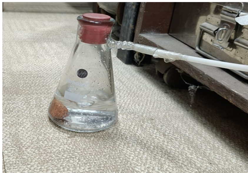
Figure 3. Water absorption test.
